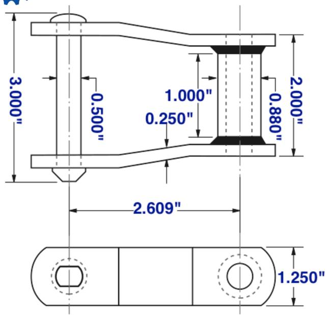
WH78 FULLY HEAT-TREATED WELDED STEEL CHAIN
